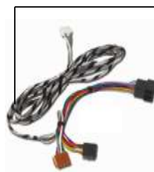
Head unit – subwoofer interconnect cable
