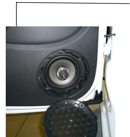
Installed speaker driver
