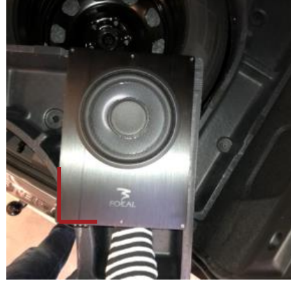
d. Part to cut to install the subwoofer.
